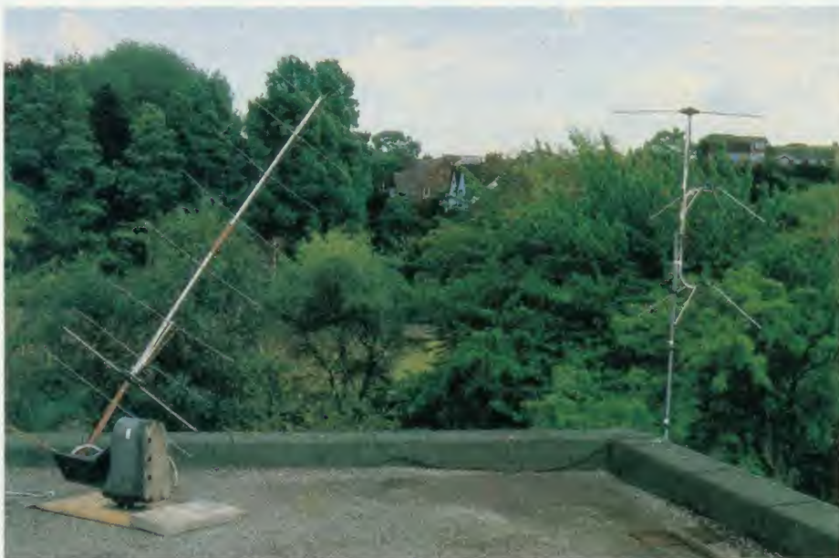
View of antennae: yagi left, NOAA right, and simple dipole
